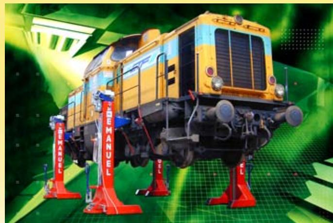
**COLONNE CON BENNA MOBILE • JACKS WITH MOVEABLE ANVILS • COLUMNAS CON UÑAS MÓVILES
