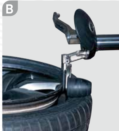
A-B. The upper BEAD BREAKER DISC and built-in plastic roller push the tyre into the rim.
