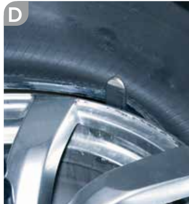
C-D. If required, the lower arm tool will help you perform this operation on particularly soft tyres.
