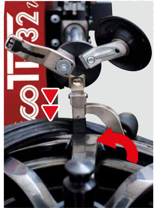
Complete MOUNTING operation facilitated by tool and built-in presser always in the same position.
