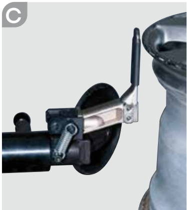
C-D. If required, the lower arm tool will help you perform this operation on particularly soft tyres.
